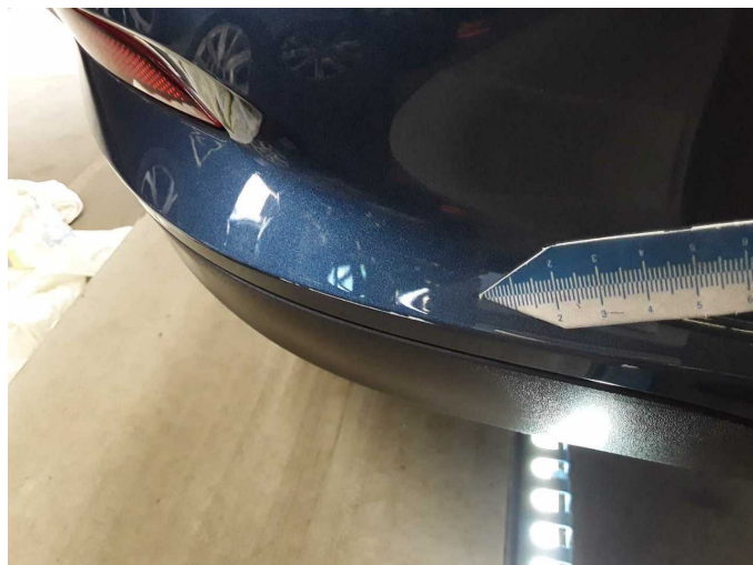
Damage 4: Rear bumper: Rear bumper - Scratch(es) - Paint
