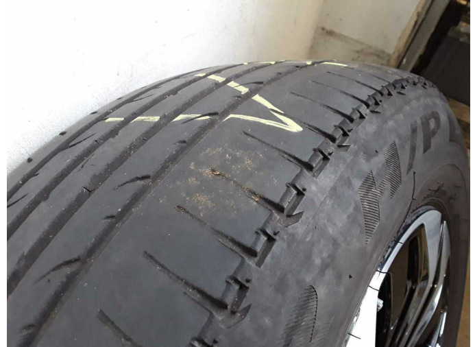
Damage 4: 2nd wheel set: 1 tyre (Außen abgefahren) - Does not meet the leasing specifications - Replace
