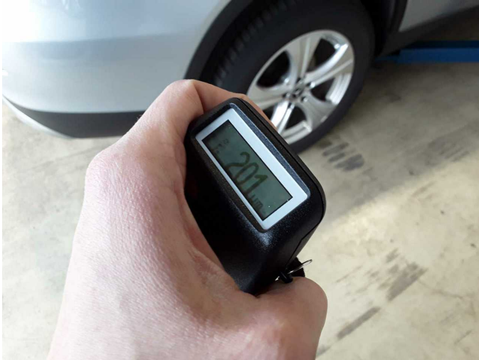
Repainting 2: Side panel - rear right side
