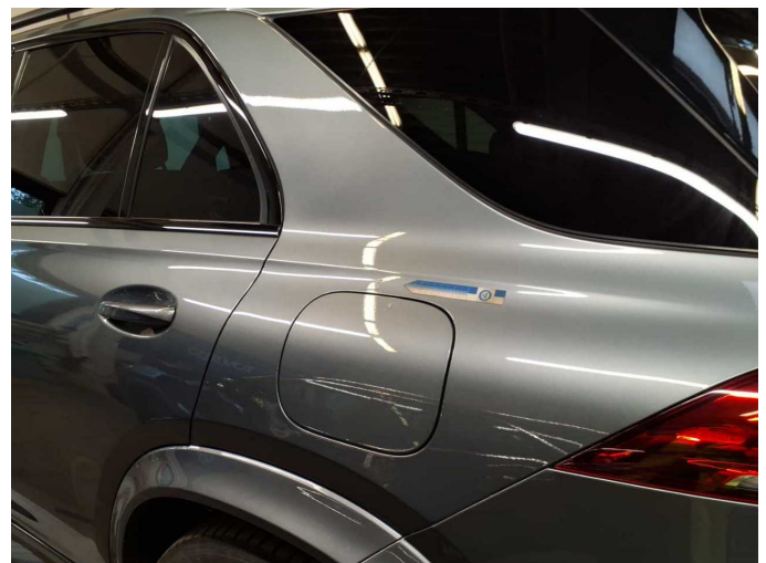
Damage 5: Side panel - rear left side: Side panel (Harzflecken-Mehrkosten möglich) - Paint defect - Conditioning
