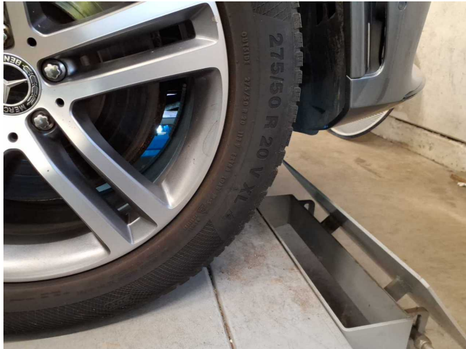
Wear and tear 1: Wheel / tyres: Tyre - front right side (nicht fahrbereit) - Broken / torn - No deduction
