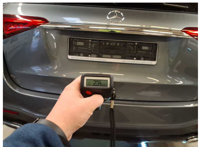
Repainting 1: Boot lid / rear door, Mudguard - right side, Bonnet, Door - front right side
