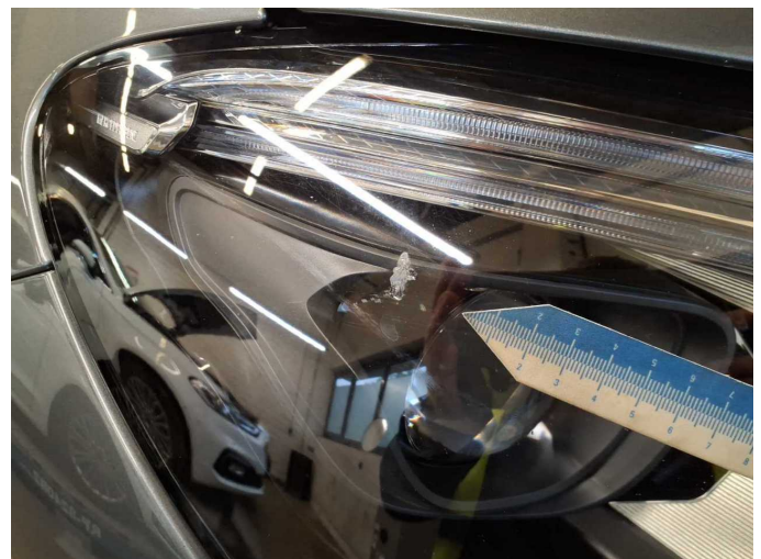
Damage 1: Headlight: Headlight - right side (Harzflecken) - Paint defect - Smart repair
