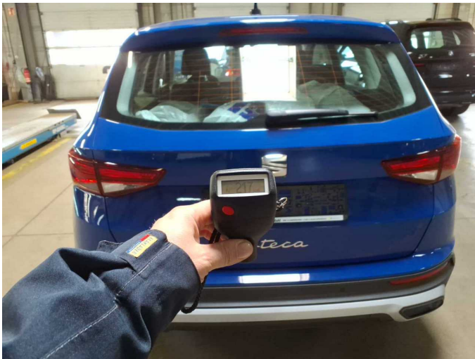
Repainting 1: Boot lid / rear door
