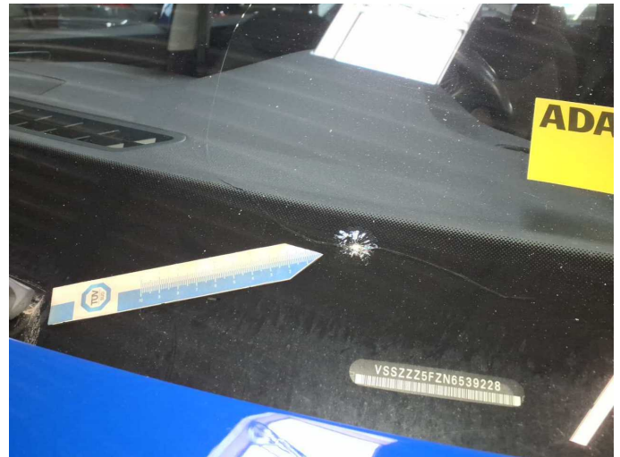
Damage 4: Vehicle glazing: Windscreen - Broken / torn - Replace
