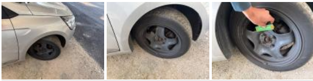
Tyre FR, Out of tolerance, Replace
