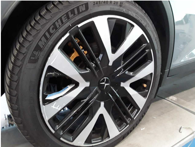
Damage 2: Wheel / tyres: Alloy rim - rear right side - Scratched - Loss in value
