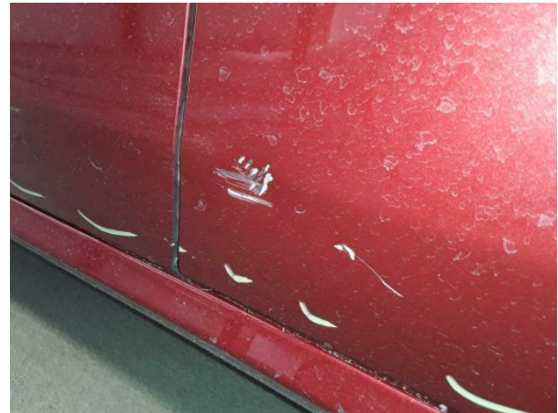
Damage #17: Mudguard - right side: Mudguard - right side - Dent / paintcoat damage - Repair and paint
