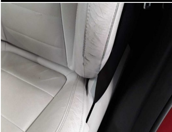
Damage #15: Seat - front: Seat cover - left side - Porous / cracke... Replace
