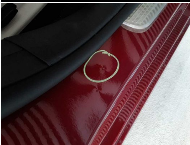
Damage #13: Sill - right side: Sill - Dent / paintcoat damage - Smart repair
