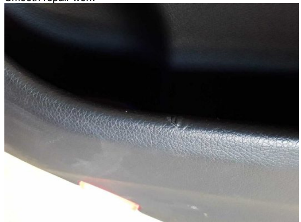
Damage #9: Trim / covers: Door trim - rear right side - Damaged - Loss in value
