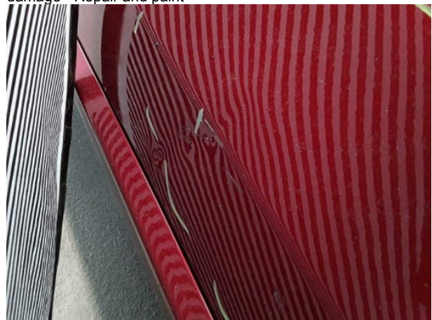
Damage #20: Door - front right side: Door - Dent / paintcoat damage - Repair and paint
