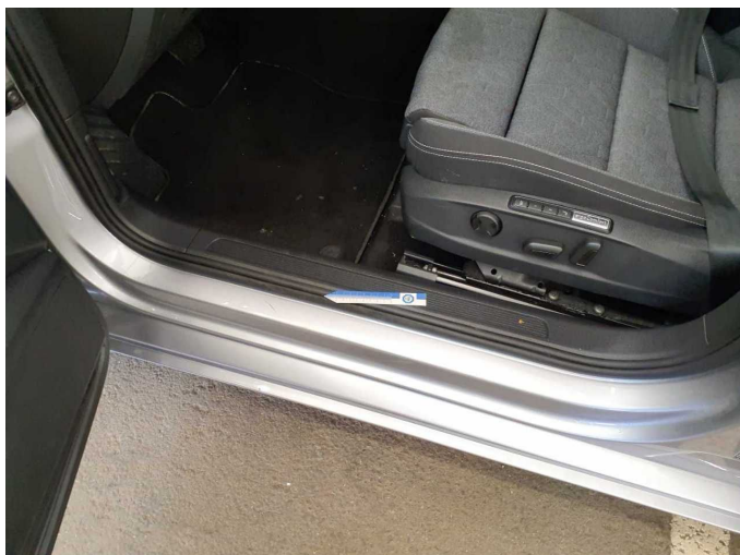
Damage 8: Door - front left side: Door seal - Porous / cracked - Replace
