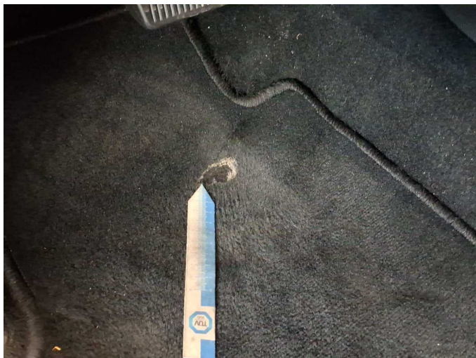
Damage 1: Trim / covers: Floor mats - Holes - Replace
