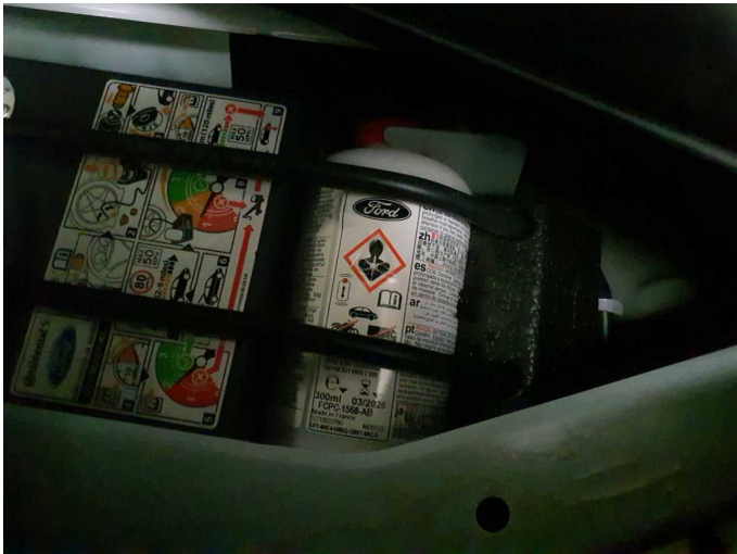
Damage 1: Equipment: Tirefit filler - Expired - Replace
