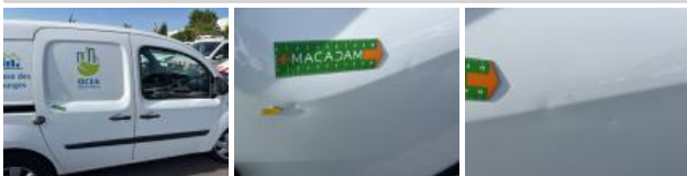
Sliding door R, Dent(s), Repair and paint (complete)
