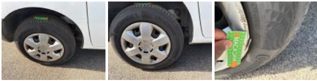
Wheel cover FR, Broken, Replace
