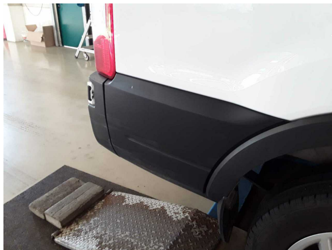
Damage 3: Side panel - rear right side: Protection strip (hinten) - Scratched - Replace
