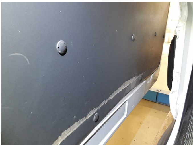
Damage 2: Sliding door, right: Trim washable - lower - Broken / torn - Replace
