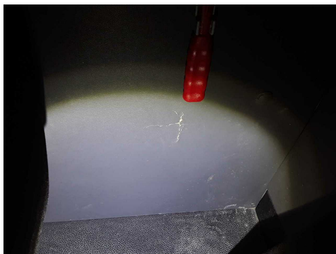
Damage 4: Side panel - rear left side: Interior trim - Broken / torn - Replace
