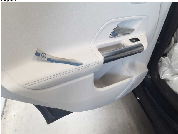
Damage #4: Trim / covers: Door trim - rear left side - Deformed - Replace
