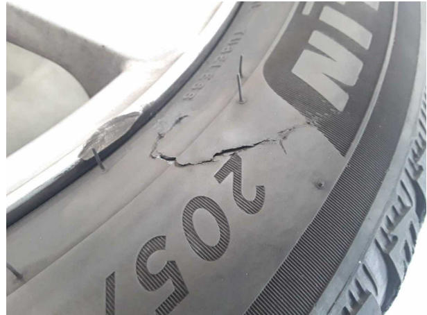
Damage #2: 2nd wheel set: 1 tyre - Broken / torn - No deduction
