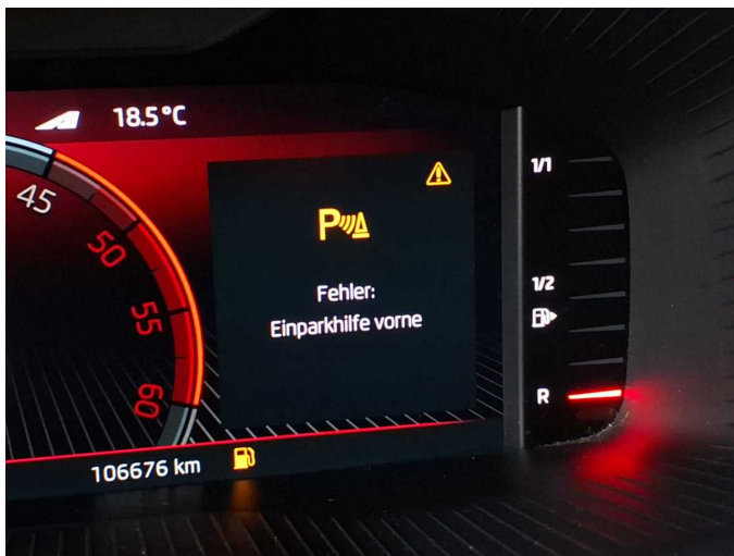
Damage 3: Electronic systems: Parking assistance - on - Perform diagnosis
