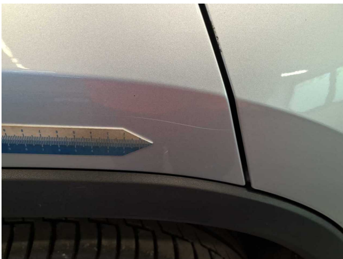
Damage 4: Side panel - rear right side: Side panel - Scratch(es) - Smart repair
