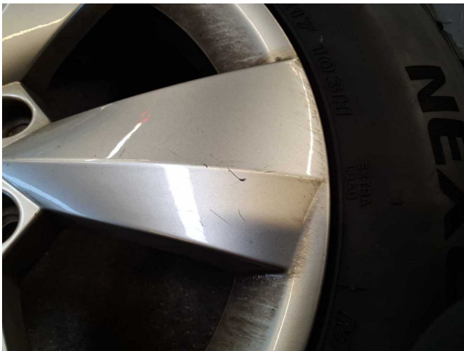
Damage 6: 2nd wheel set: 1 alloy rim - Scratch(es) - Smart repair
