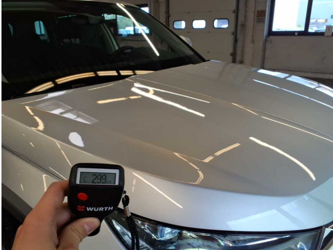
Repainting 1: Mudguard - right side, Bonnet, Door - rear right side, Door - front right side
