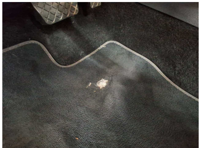
Damage 2: Trim / covers: Floor mats - Holes - Replace
