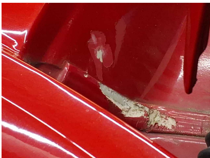
Damage 7: Roof: Roof - Scratched - Smart repair
