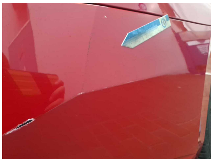
Damage 9: Rear bumper: Rear bumper - Scratch(es) - Paint
