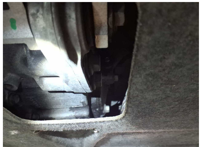
Damage 2: Gearbox: Gearbox - Leaking - Perform diagnosis
