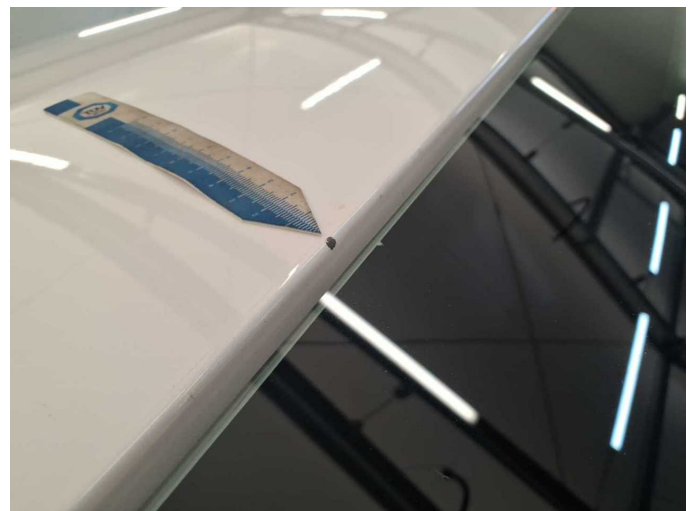
Damage 4: Roof: Roof - Stone chips - Paint
