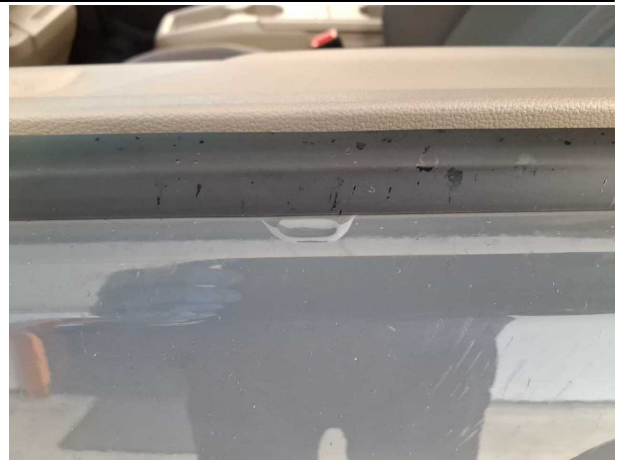
Damage #5: Door - front left side: Door - Paint defect - Repair and paint
