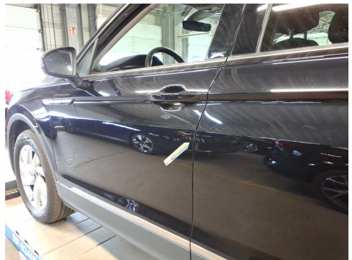
Wear and tear 4: Door - front left side: Door edge - Scratch(es) - Smart repair
