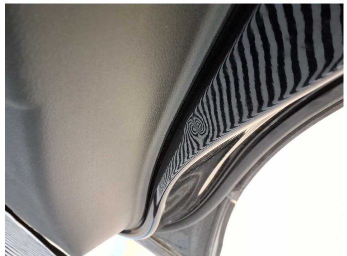
Damage 3: Door - rear right side: Door (Innen) - dent(s) - Smooth repair work
