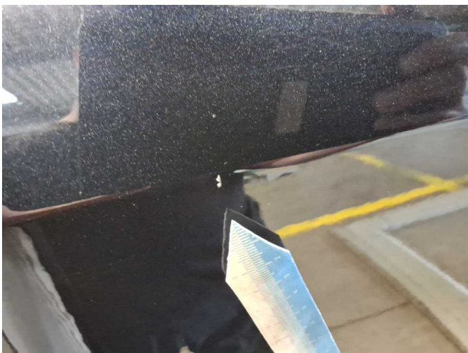
Damage 7: Door - front right side: Door - Dent / paintcoat damage - Smart repair
