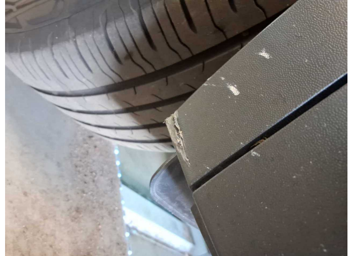
Damage 8: Mudguard - right side: Wheel well extension (Materialabtrag) - Scratched - Replace
