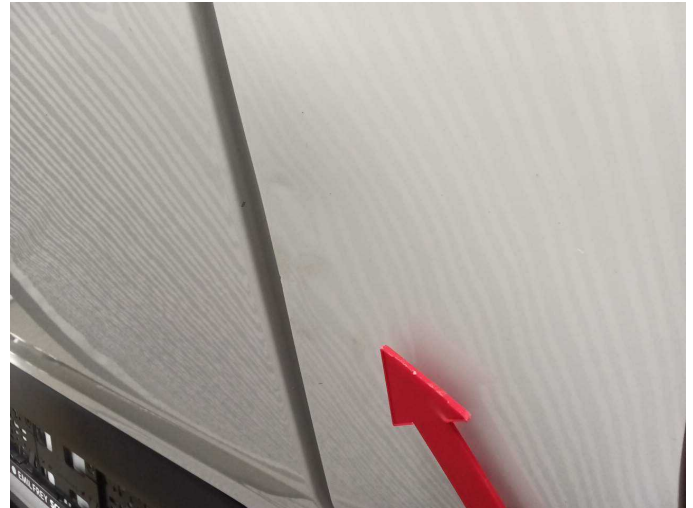
Damage 17: Boot lid / rear door: Rear door - right side - Dent / paintcoat damage - Repair and paint
