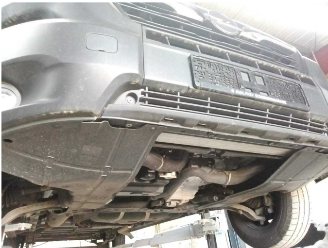
Damage 14: Front bumper: Front bumper - Scratched - Replace
