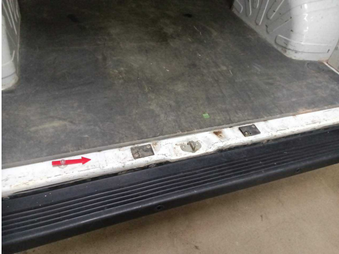
Damage 7: Rear of vehicle: Rear panel - Scratched - Smart repair
