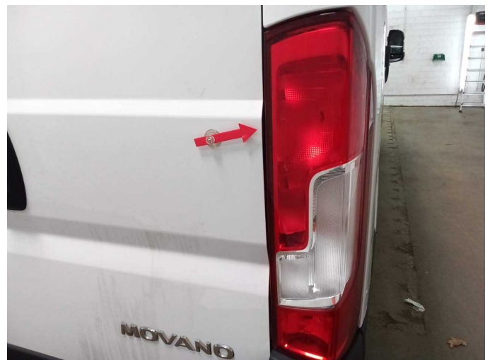
Damage 11: Tail light: Tail lamp - right side - Scratch(es) - Replace
