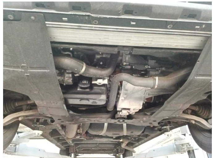
Damage 12: Engine: Engine cowling - lower - Missing - Replace
