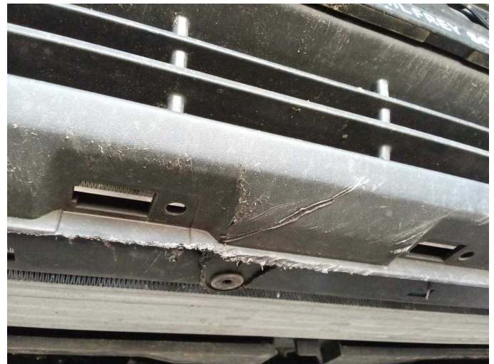
Damage 14: Front bumper: Front bumper - Scratched - Replace
