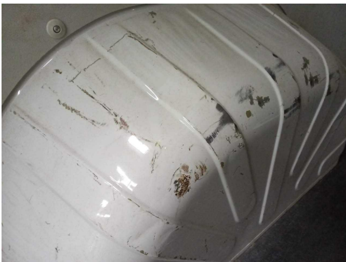
Damage 4: Interior: Interior (Laderaum) - Dent / paintcoat damage - Loss in value
