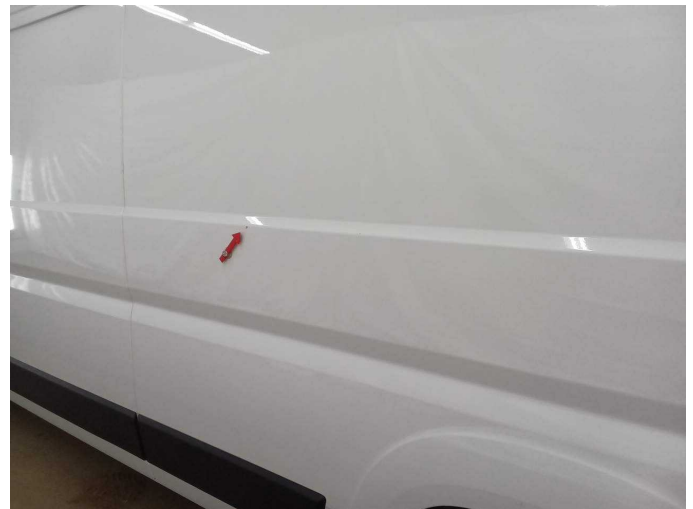
Damage 10: Side panel - rear left side: Side panel - Dent / paintcoat damage - Smart repair
