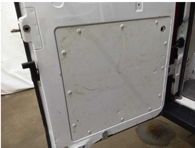
Damage 13: Trim / covers: Boot lid - interior trim (Hecktür links & rechts) - Scratched - Replace
