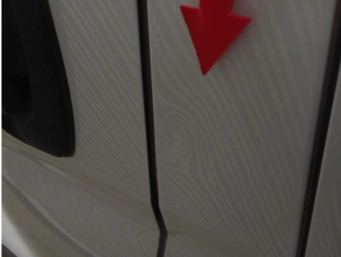
Damage 3: Body: B-pillar - right side - dent(s) - Smooth repair work
