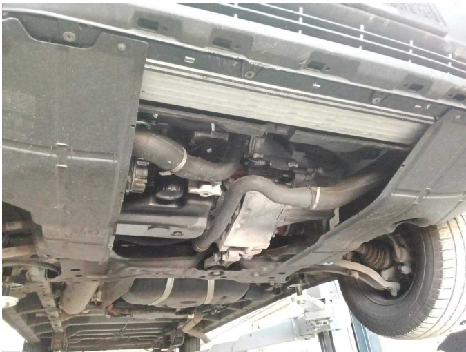
Damage 12: Engine: Engine cowling - lower - Missing - Replace
