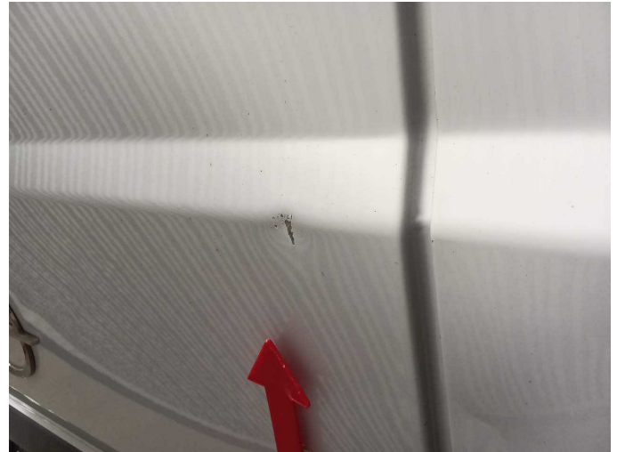
Damage 16: Boot lid / rear door: Rear door - left side - Dent / paintcoat damage - Repair and paint
