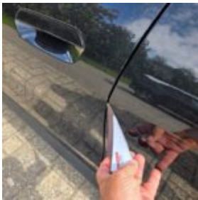
Damage Type Door-edge chipped
