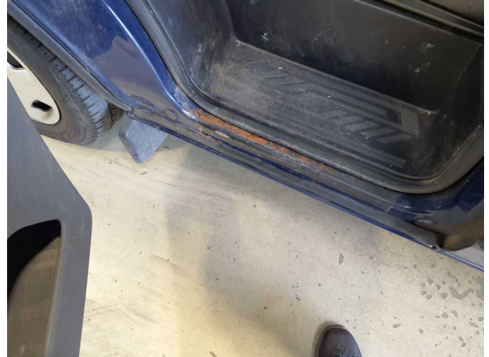
Damage 8: Sill - left side: Sill - Corrosion - Repair and paint
