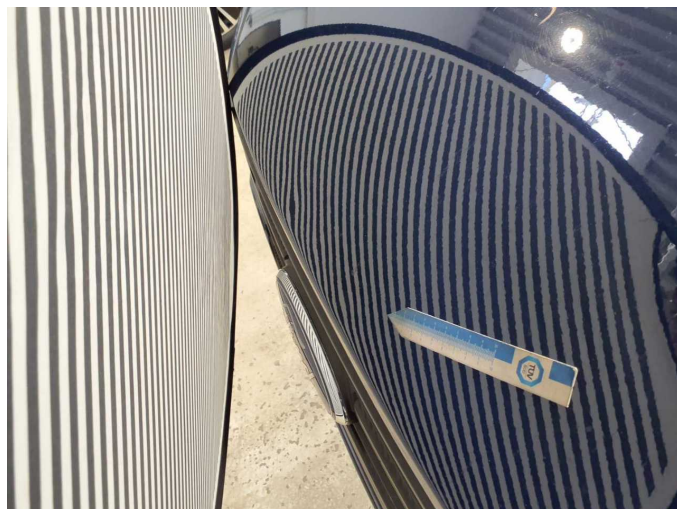
Damage 21: Bonnet: Bonnet - Dent / paintcoat damage - Repair and paint
