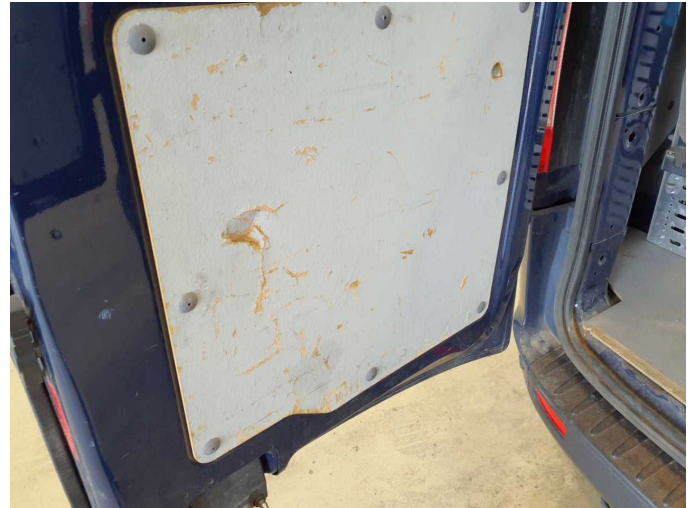
Damage 11: Trim / covers: Trim / covers (Heck tür links und rechts) - Broken / torn - Replace
