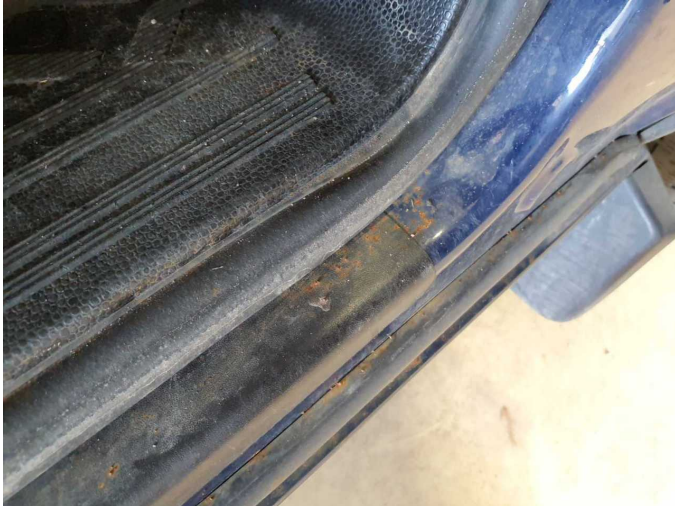
Damage 7: Sill - right side: Sill - Corrosion - Repair and paint
