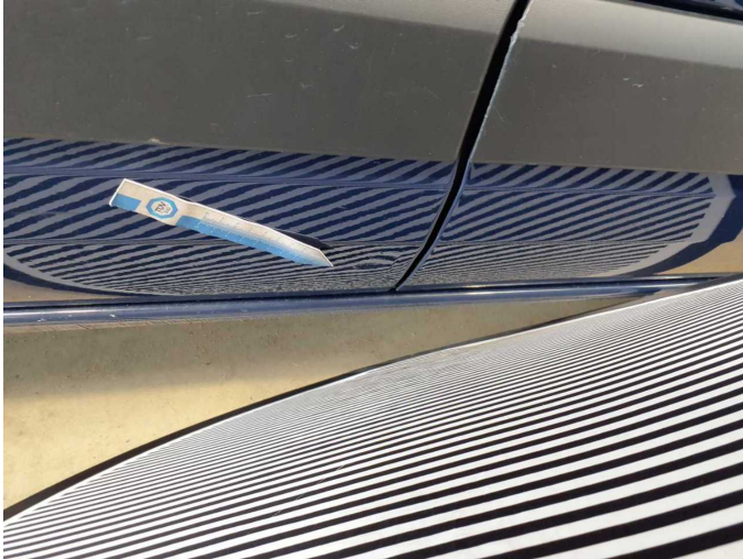
Damage 19: Sliding door, right: Sliding door (Einschlüsse und unförmig) - Unprofessionally repaired - Repair and paint
