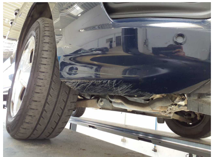
Damage 20: Front bumper: Front bumper - Scratch(es) - Paint
