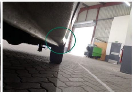
Schweller / Links / Delle
