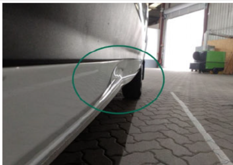
Schweller / Links / Delle
