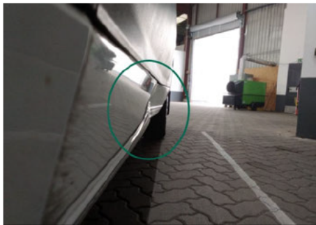
Schweller / Links / Delle
