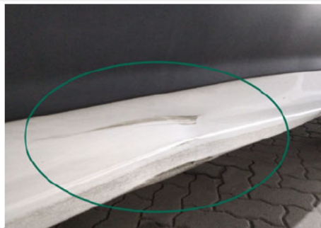
Schweller / Links / Delle
