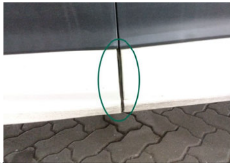
Schweller / Links / Delle
