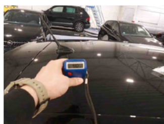
Paint thickness Roof
