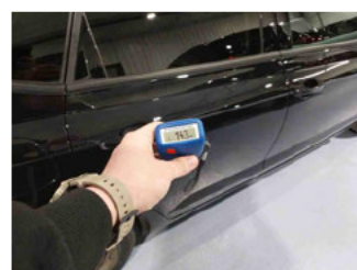
Paint thickness Door RR
