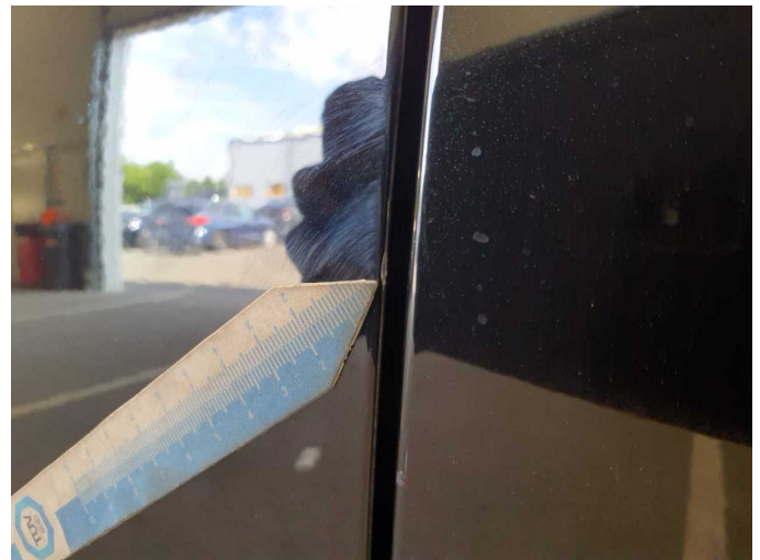
Wear and tear 4: Door - front left side: Door edge - Scratch(es) - No deduction
