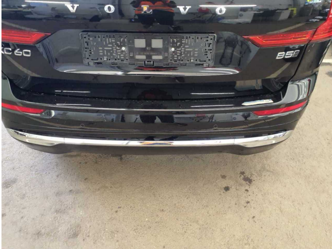
Damage 2: Rear bumper: Rear bumper - Scratched - Smart repair
