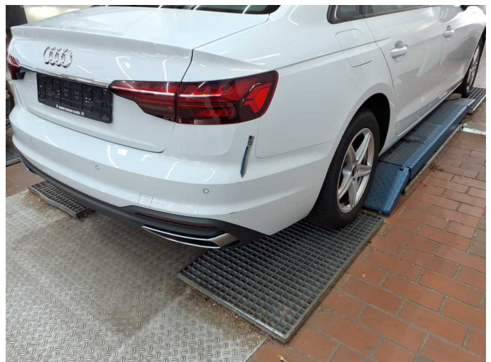
Damage 1: Rear bumper: Rear bumper - Scratch(es) - Paint
