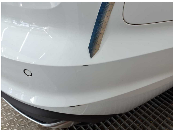
Damage 1: Rear bumper: Rear bumper - Scratch(es) - Paint
