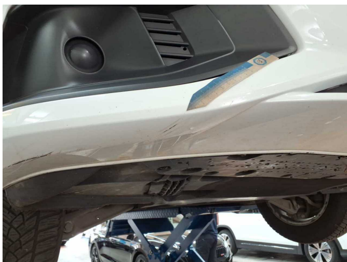
Damage 2: Front bumper: Front bumper - Scratch(es) - Paint
