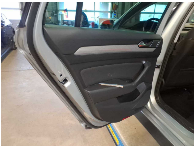
Damage 5: Door - rear left side: Door handle - inside - Broken / torn - Smart repair
