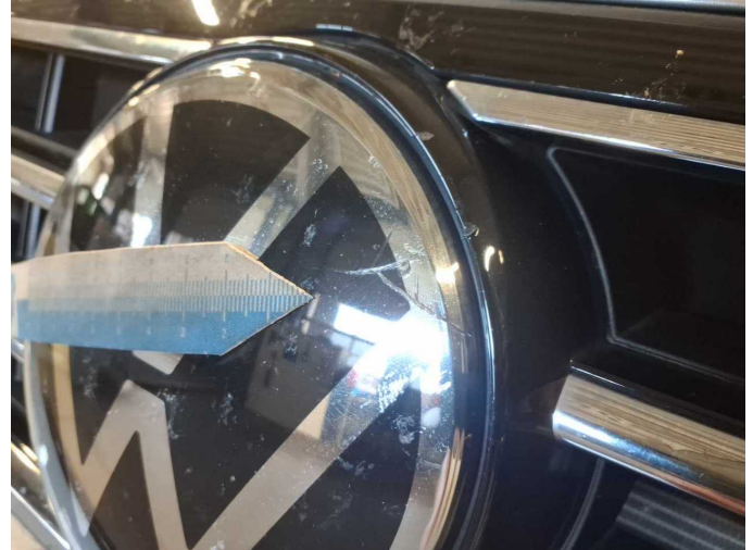
Damage 6: Bonnet: Emblem - Broken / torn - Replace
