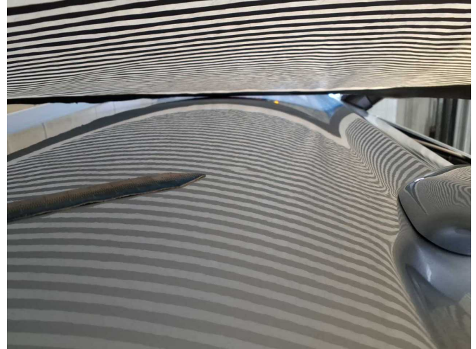
Damage 2: Door - front left side: Door - dent(s) - Smooth repair work
