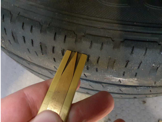
Damage 4: 2nd wheel set: 2 tyres (Sommerreifen Profiltiefe <math>< 2\text{mm}</math>) - Worn - Replace
