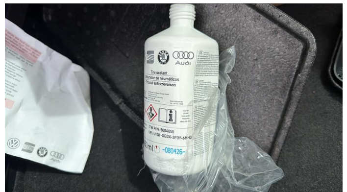
Damage 1: Equipment: Tirefit filler - Expired - Replace
