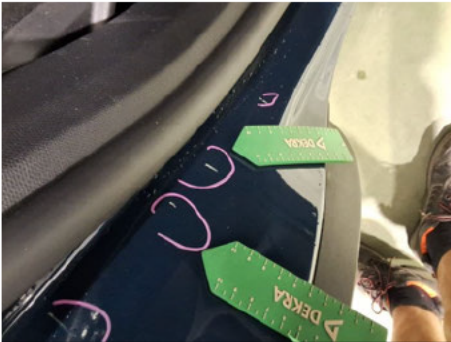
Door sill / Interior Back Right / Scratched
