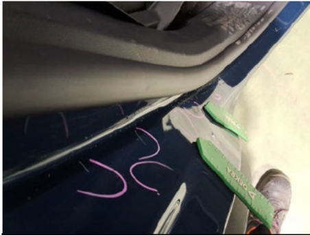
Door sill / Interior Back Right / Scratched
