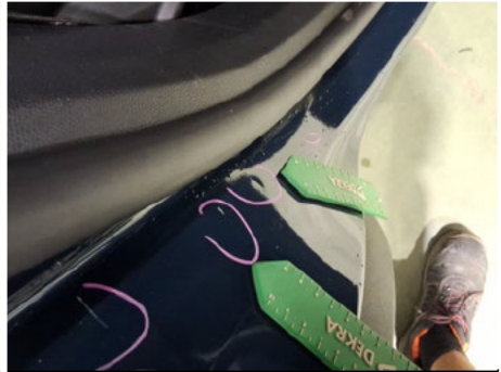
Door sill / Interior Back Right / Scratched
