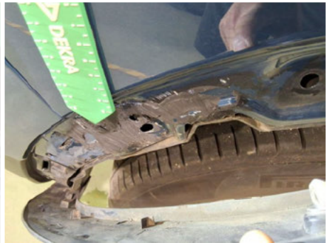
Wing extension moulding / Back Right / Broken
