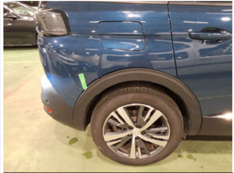
Wing extension moulding / Back Right / Broken
