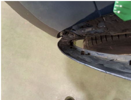
Wing extension moulding / Back Right / Broken
