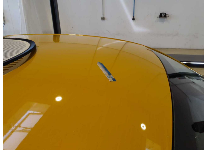
Damage 1: Roof: Roof - dent(s) - Smooth repair work
