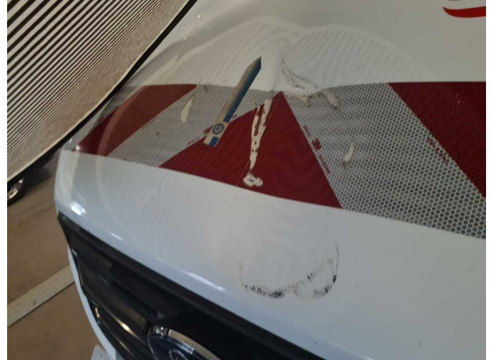
Damage 6: Bonnet: Bonnet - Dent / paintcoat damage - Replace
