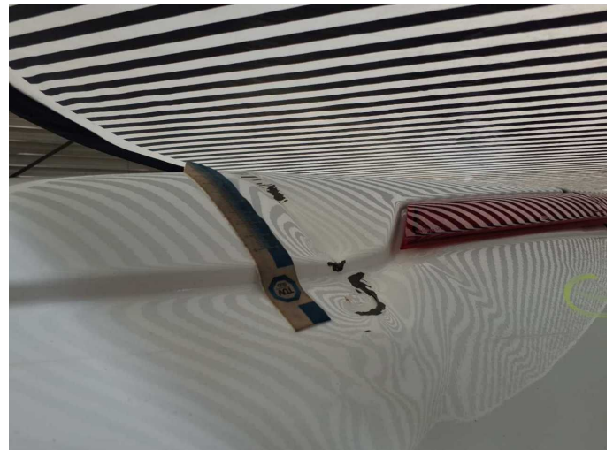
Damage 8: Boot lid / rear door: Rear door - left side (Inkl. Folie) - Dent / paintcoat damage - Replace
