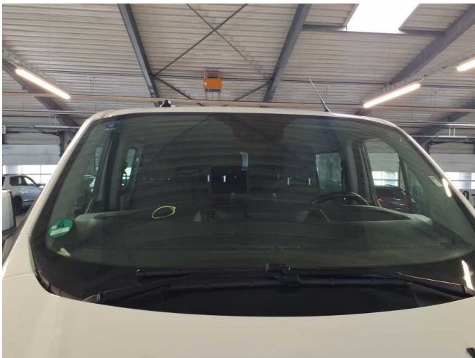
Damage 7: Vehicle glazing: Windscreen - Unprofessionally repaired - Replace
