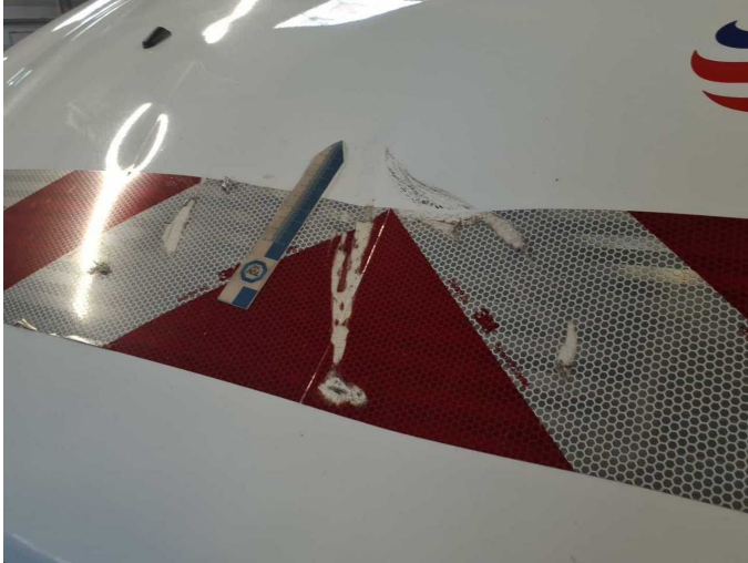
Damage 6: Bonnet: Bonnet - Dent / paintcoat damage - Replace
