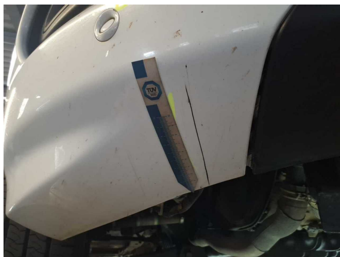
Damage 5: Front bumper: Front bumper - Scratch(es) - Paint
