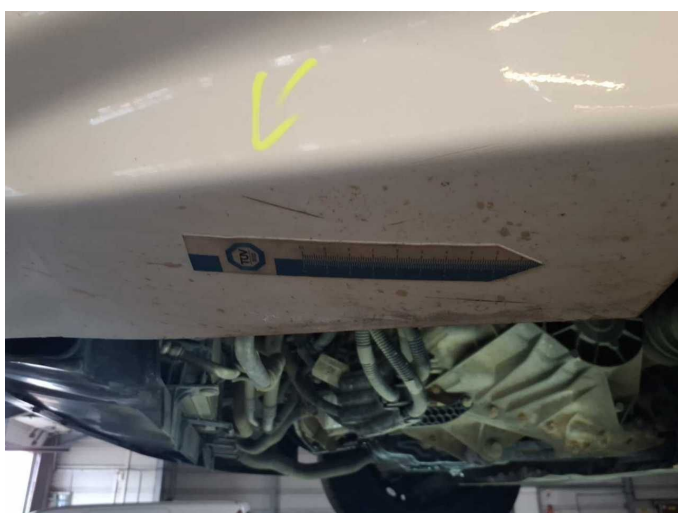
Damage 5: Front bumper: Front bumper - Scratch(es) - Paint
