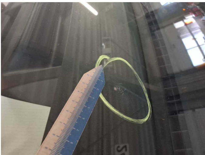
Damage 7: Vehicle glazing: Windscreen - Unprofessionally repaired - Replace
