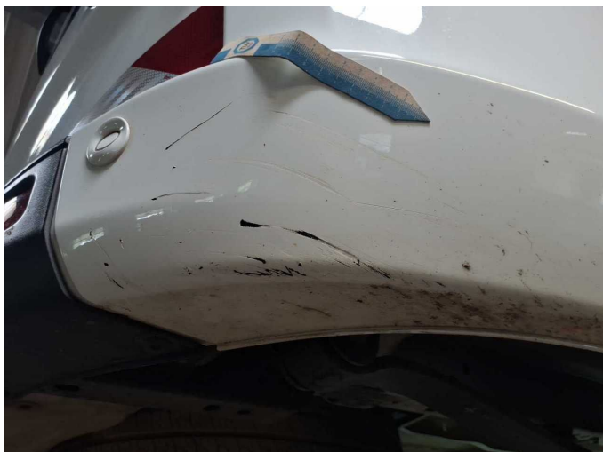
Damage 4: Rear bumper: Rear bumper - Scratched - Paint
