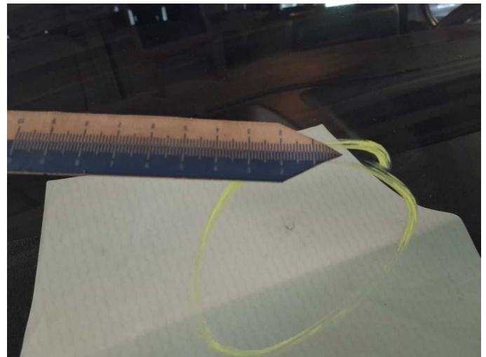
Damage 7: Vehicle glazing: Windscreen - Unprofessionally repaired - Replace
