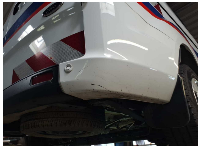
Damage 4: Rear bumper: Rear bumper - Scratched - Paint
