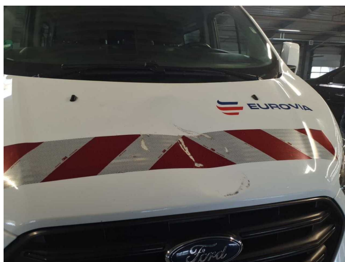
Damage 6: Bonnet: Bonnet - Dent / paintcoat damage - Replace
