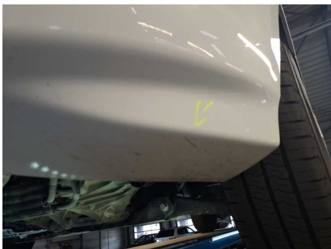
Damage 5: Front bumper: Front bumper - Scratch(es) - Paint
