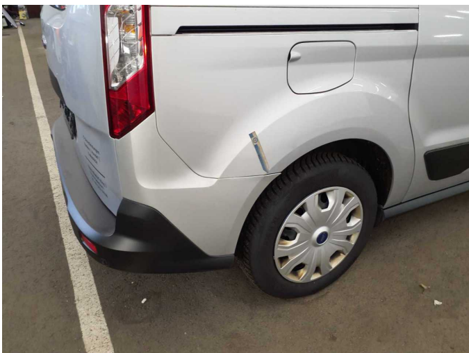
Damage 2: Rear bumper: Rear bumper - Malposition - Un- / install
