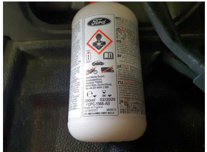
Damage 1: Equipment: Tirefit filler - Expired - Replace
