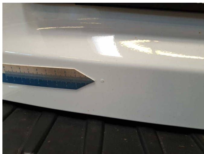
Damage 6: Boot lid / rear door: Rear door - left side (Korrosion) - Paint defect - Paint
