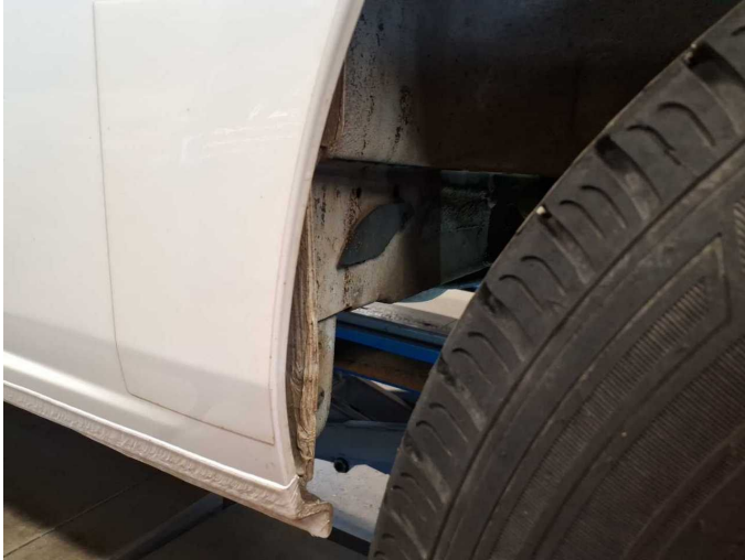
Damage 2: Side panel - rear left side: Mud flap - Missing - Replace
