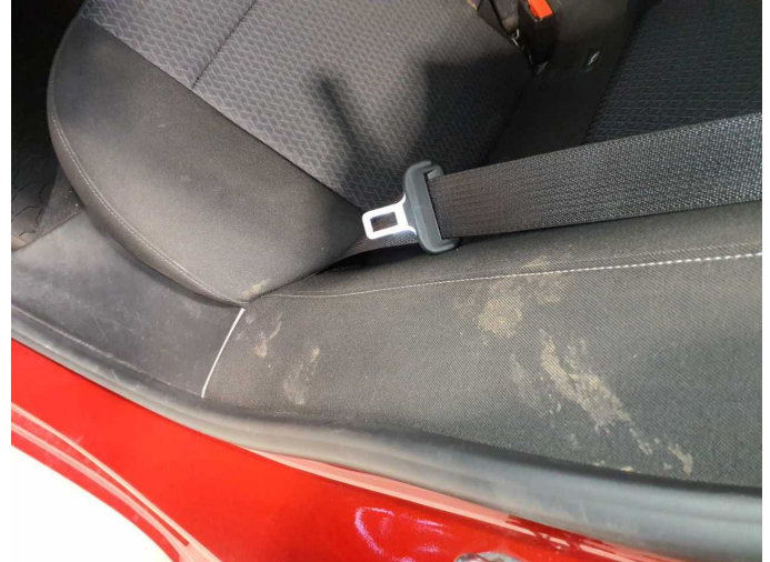
Damage 6: Seat - rear: Upholstery - Soiled - Clean
