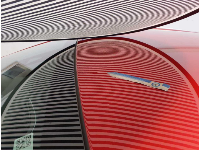
Damage 23: Roof: Roof (Anätzung) - Paint defect - Paint
