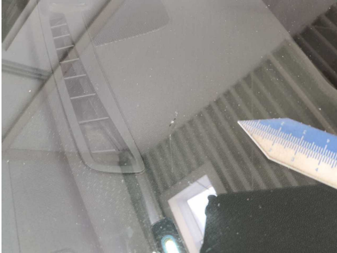
Damage 20: Vehicle glazing: Windscreen - Broken / torn - Replace
