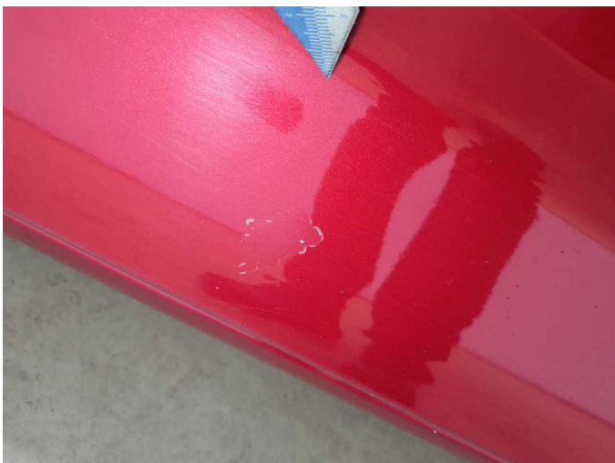
Damage 19: Door - front right side: Door - Dent / paintcoat damage - Repair and paint
