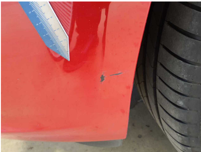
Damage 22: Front bumper: Front bumper (Gestaucht) - Dent / paintcoat damage - Replace
