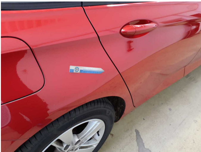
Damage 7: Side panel - rear right side: Side panel - dent(s) - Smooth repair work
