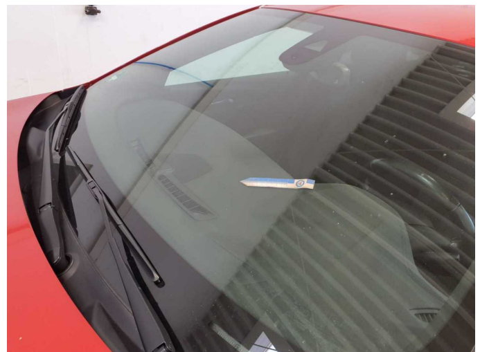
Damage 20: Vehicle glazing: Windscreen - Broken / torn - Replace
