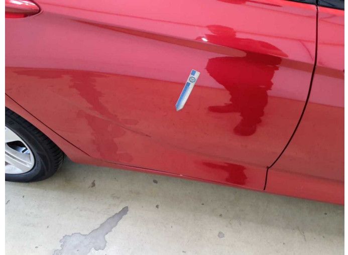
Damage 12: Door - rear right side: Door - Scratch(es) - Loss in value
