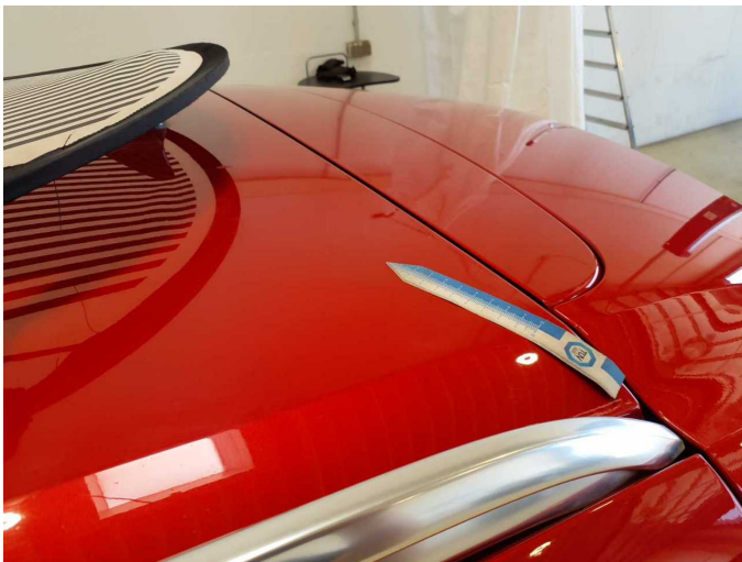
Damage 23: Roof: Roof (Anätzung) - Paint defect - Paint
