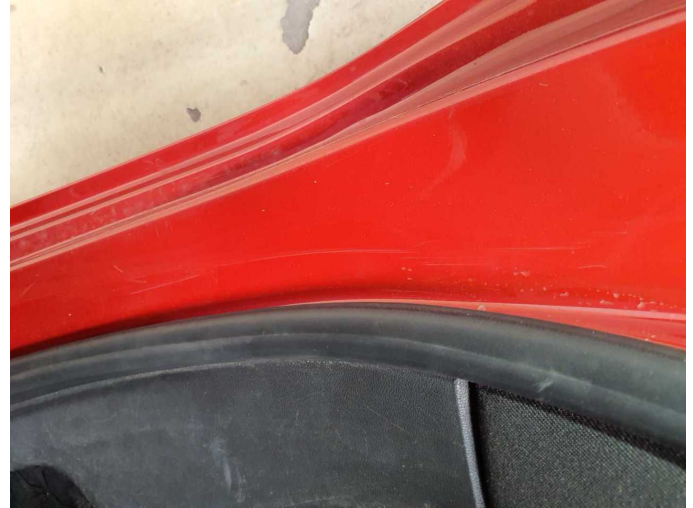
Damage 9: Side panel - rear right side: Sill - Scratch(es) - Smart repair
