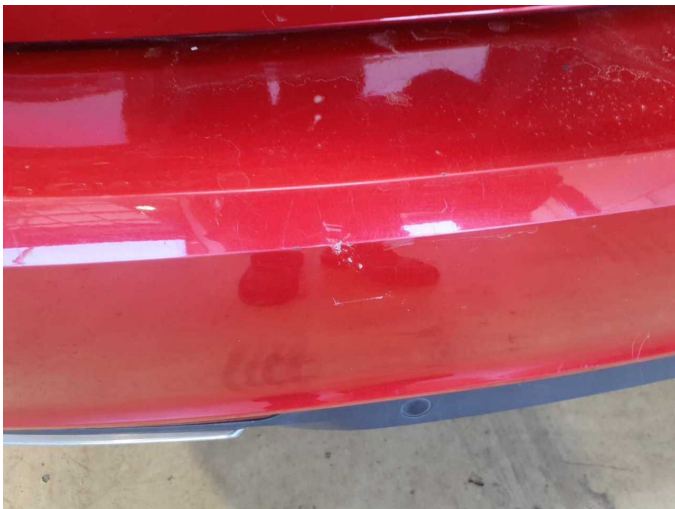
Damage 16: Rear bumper: Rear bumper - Dent / paintcoat damage - Repair and paint
