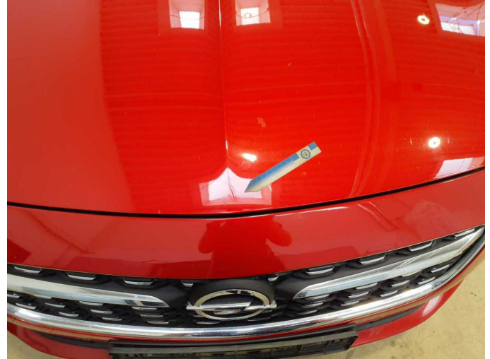
Damage 21: Bonnet: Bonnet (Lack löst sich) - Paint defect - Repair and paint
