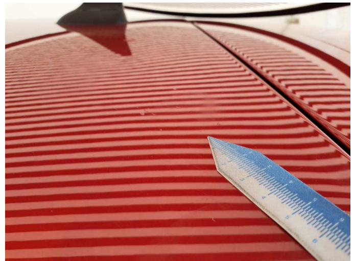
Damage 23: Roof: Roof (Anätzung) - Paint defect - Paint
