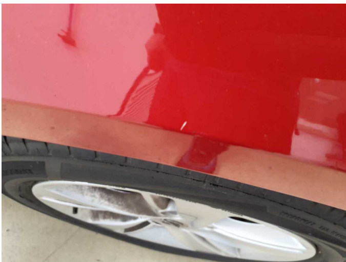
Damage 10: Mudguard - right side: Mudguard - right side - Dent / paintcoat damage - Smart repair
