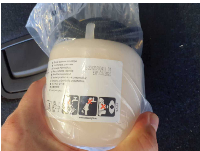
Damage 1: Equipment: Tirefit filler - Expired - Replace
