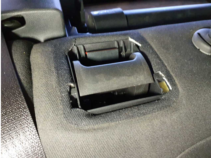
Damage 2: Seat - rear: Lever seat adjustment - Broken / torn - Replace
