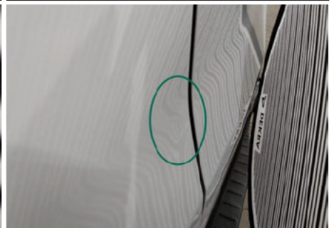
Heckklappe / Kofferraumtür / Hinten Links / Delle
