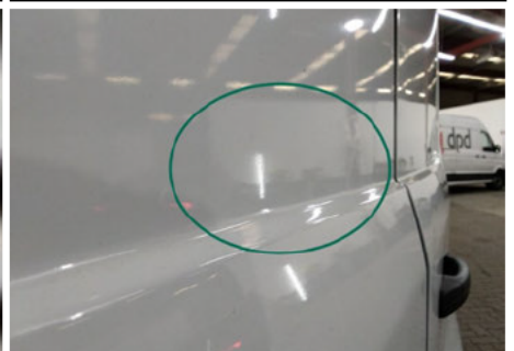
Heckklappe / Kofferraumtür / Hinten Links / Delle
