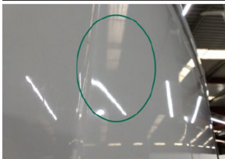
Heckklappe / Kofferraumtür / Hinten Links / Delle
