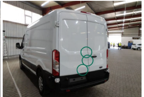
Heckklappe / Kofferraumtür / Hinten Links / Delle
