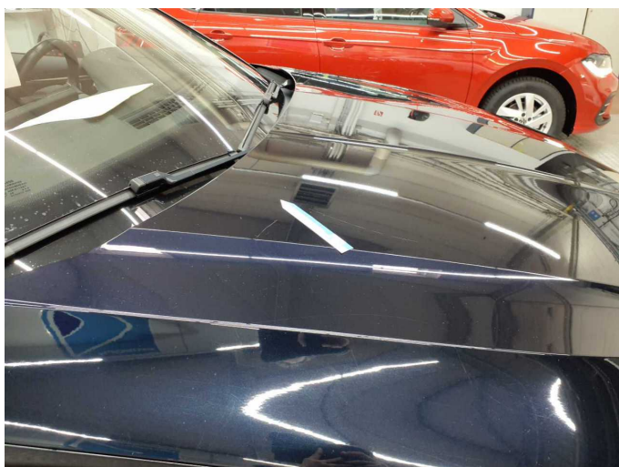
Damage 14: Bonnet: Bonnet - Dent / paintcoat damage - Paint
