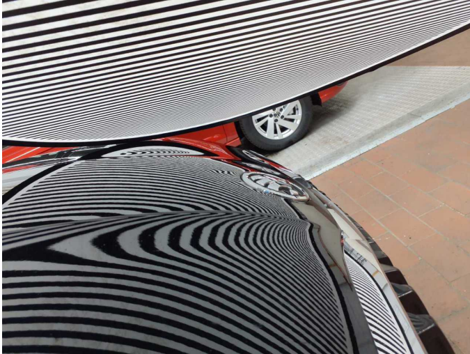
Damage 14: Bonnet: Bonnet - Dent / paintcoat damage - Paint
