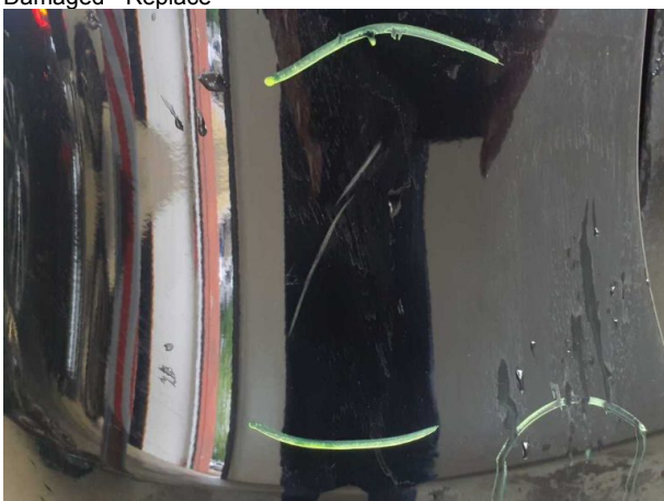
Damage #5: Rear bumper: Rear bumper - Scratched - Paint
