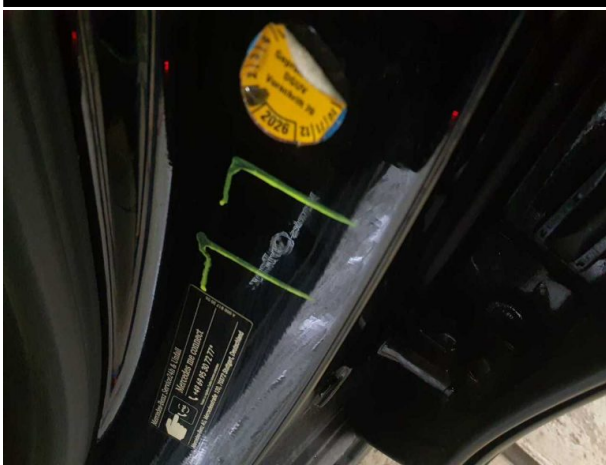
Damage #3: Sill - left side: Sill - Dent / paintcoat damage - Smart repair
