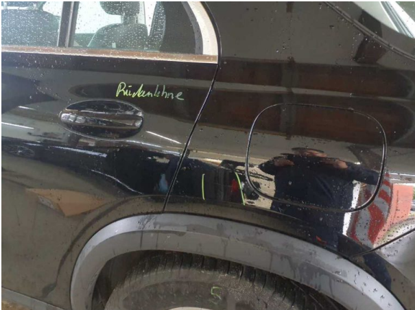
Damage #1: Side panel - rear left side: Side panel - Scratched - Cover / polish
