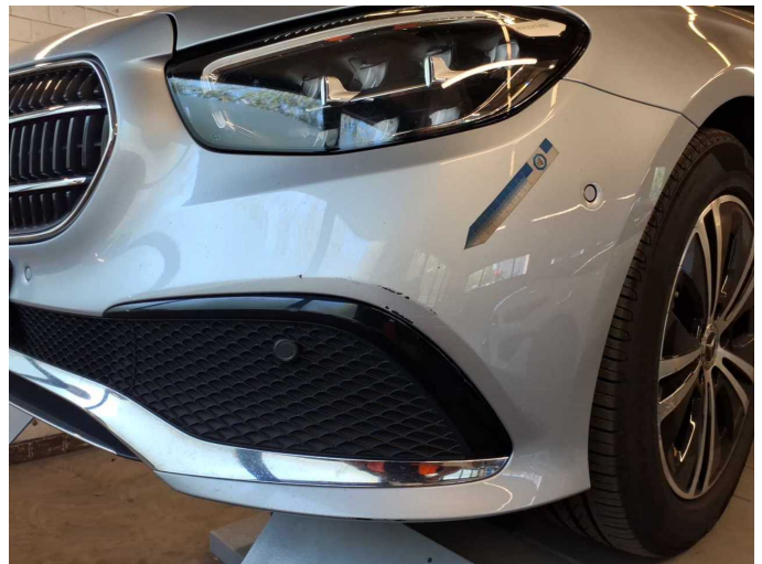
Damage 6: Front bumper: Front bumper - Scratched - Paint
