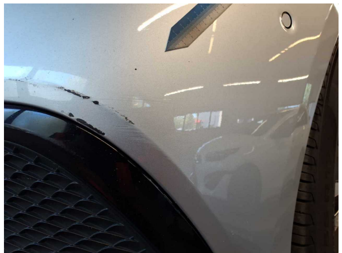
Damage 6: Front bumper: Front bumper - Scratched - Paint
