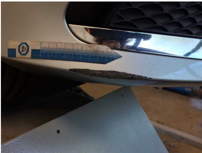
Damage 6: Front bumper: Front bumper - Scratched - Paint
