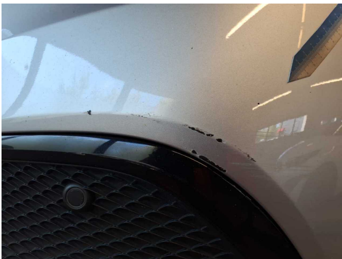
Damage 6: Front bumper: Front bumper - Scratched - Paint
