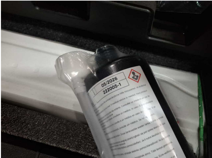
Damage 2: Equipment: Tirefit filler - Expired - Replace
