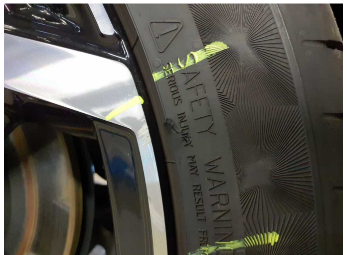
Damage 1: Wheel / tyres: Tyre - rear right side (nicht fahbereit) - Porous / cracked - Replace
