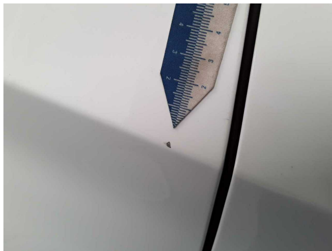
Damage 7: Door - rear right side: Door - Stone chips - Smart repair
