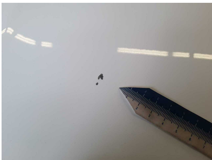
Damage 10: Bonnet: Bonnet - Stone chips - Paint
