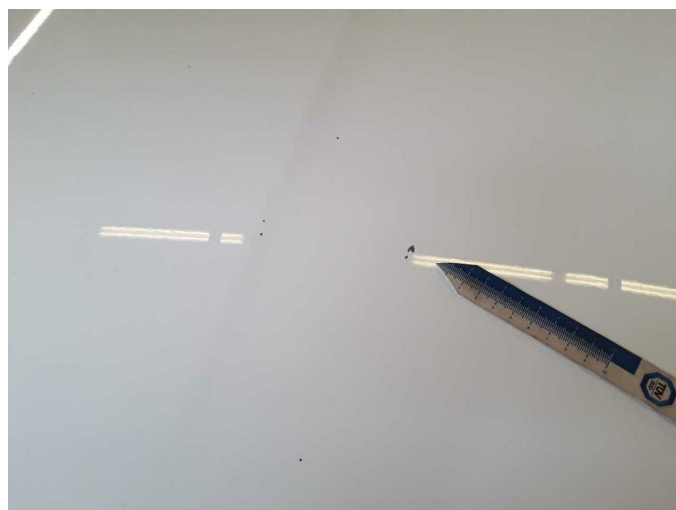
Damage 10: Bonnet: Bonnet - Stone chips - Paint
