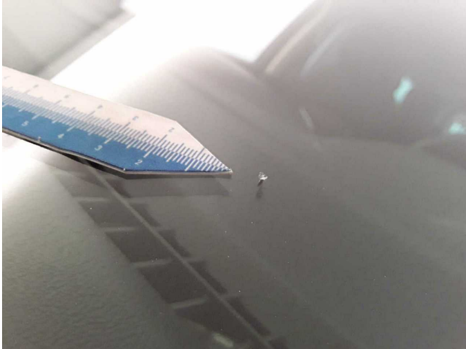
Damage 11: Vehicle glazing: Windscreen (Rissbildung) - Broken / torn - Replace
