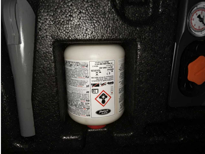
Damage 1: Equipment: Tirefit filler - Expired - Replace
