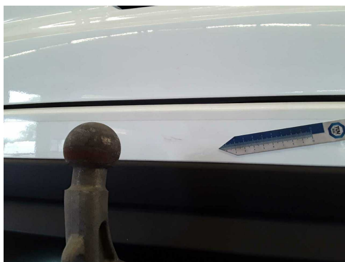
Damage 8: Rear bumper: Rear bumper - Dent / paintcoat damage - Repair and paint
