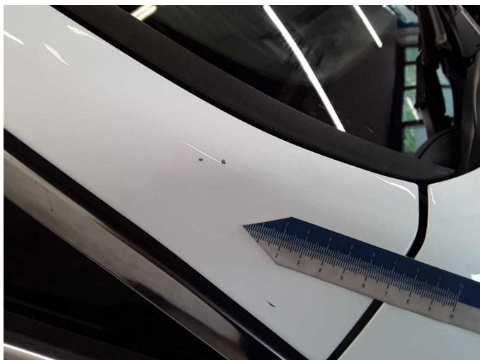
Damage 6: Roof: Roof rail - right side - Stone chips - Smart repair
