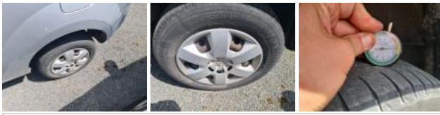
Tyre RR, Out of tolerance, Replace
