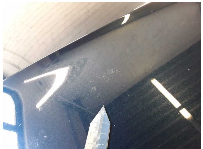
Damage 5: Bonnet: Bonnet (Vogelkot) - Paint defect - Paint
