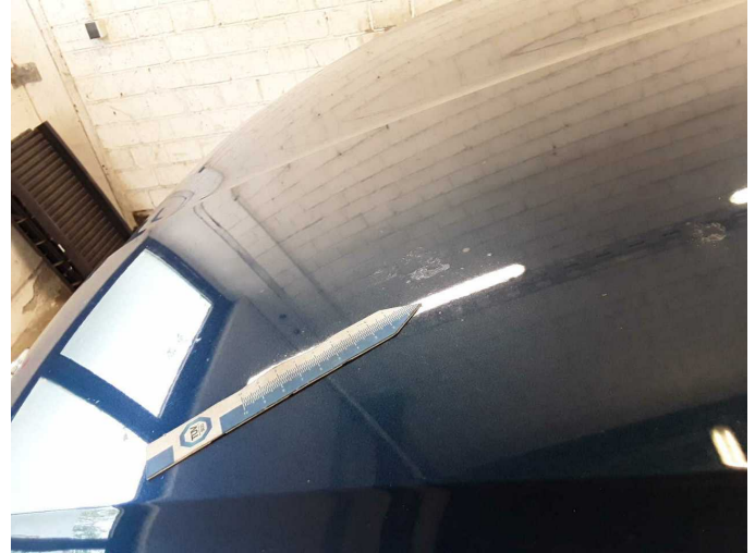
Damage 5: Bonnet: Bonnet (Vogelkot) - Paint defect - Paint
