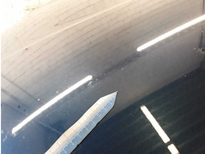
Damage 5: Bonnet: Bonnet (Vogelkot) - Paint defect - Paint
