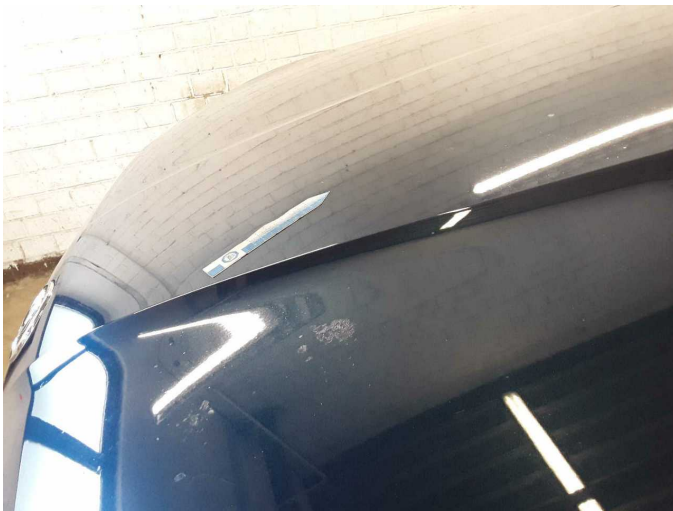
Damage 5: Bonnet: Bonnet (Vogelkot) - Paint defect - Paint
