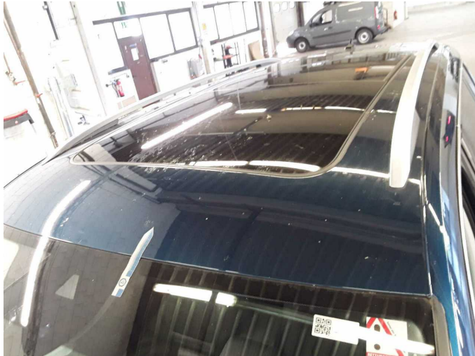
Damage 7: Roof: Roof (Vogelkot eingebrannt) - Paint defect - Paint
