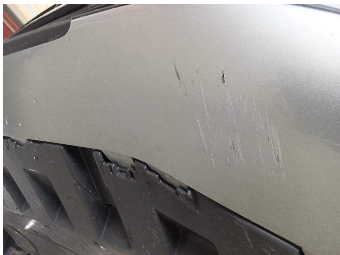
Damage 1: Front bumper: Front bumper - Scratch(es) - Paint
