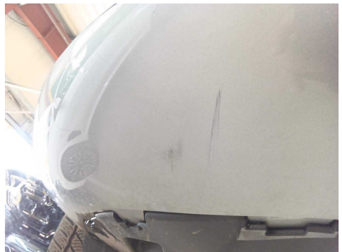
Damage 1: Front bumper: Front bumper - Scratch(es) - Paint
