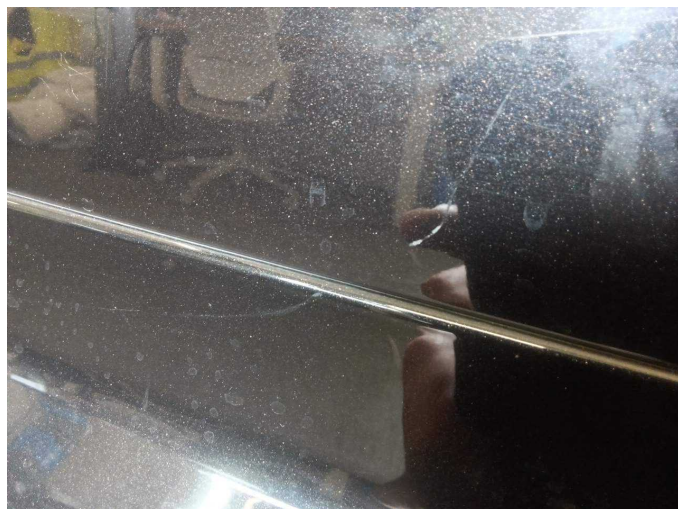
Damage 2: Rear bumper: Rear bumper - Scratch(es) - Paint
