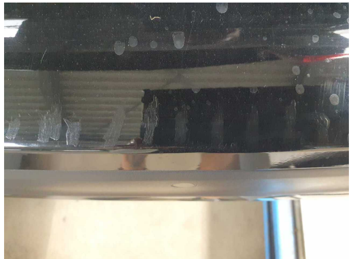
Damage 8: Rear bumper: Rear bumper - Paint defect - Repair and paint
