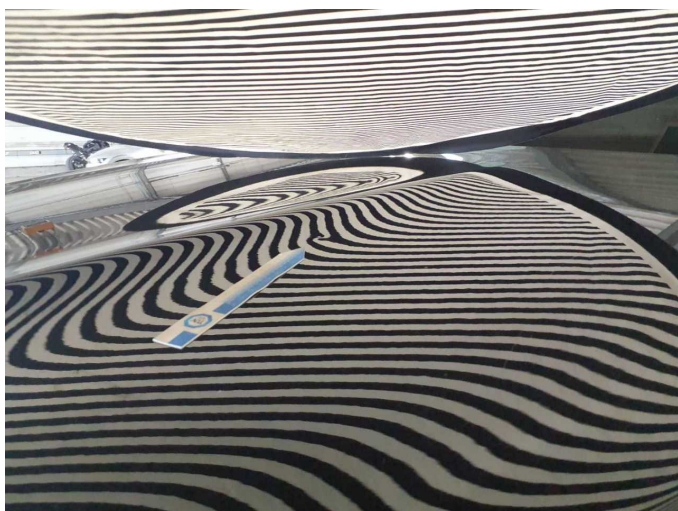
Damage 2: Bonnet: Bonnet - dent(s) - Smooth repair work
