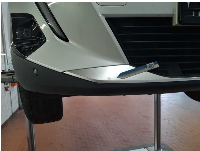
Damage 4: Trim / covers: Brightware / decorative strip (Stoßfänger vorne) - Scratch(es) - Replace
