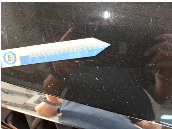
Damage 9: Bonnet: Bonnet - Stone chips - Paint
