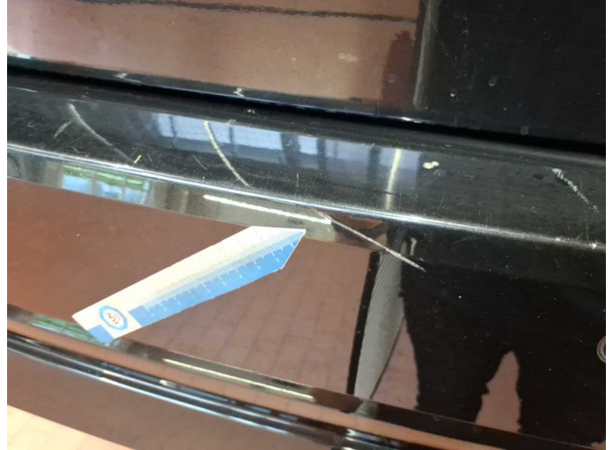
Damage 8: Rear bumper: Rear bumper - Scratch(es) - Paint
