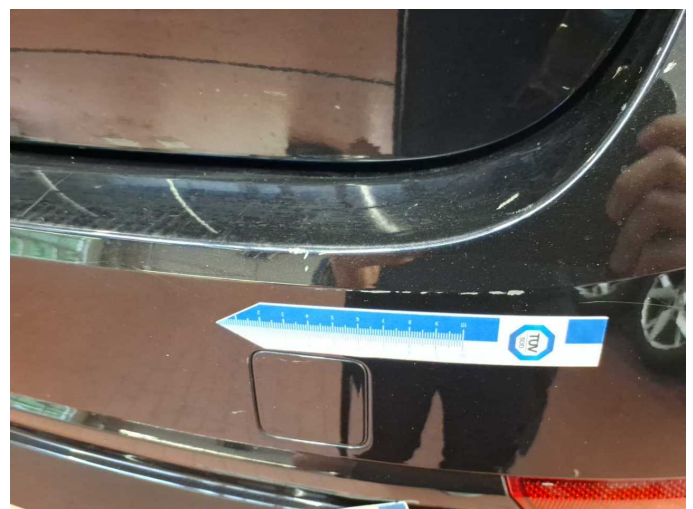
Damage 8: Rear bumper: Rear bumper - Scratch(es) - Paint
