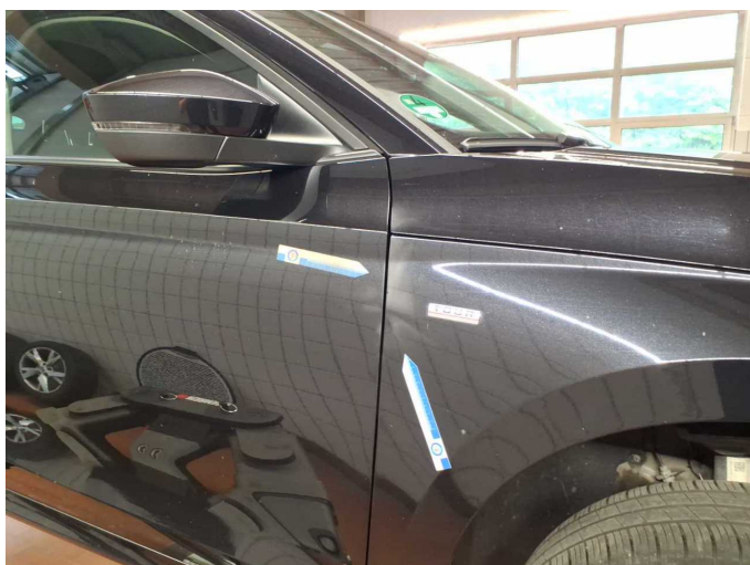
Damage 3: Body: Body (Lacknebel) - Paint defect - Conditioning
