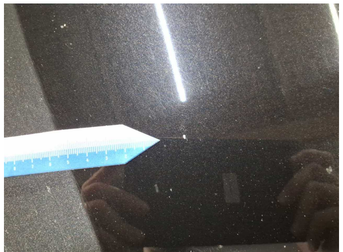
Damage 9: Bonnet: Bonnet - Stone chips - Paint
