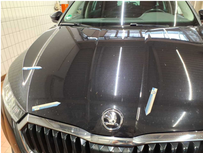
Damage 9: Bonnet: Bonnet - Stone chips - Paint
