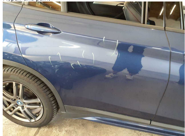
Damage #2: Door - rear right side: Door - dent(s) - Repair and paint
